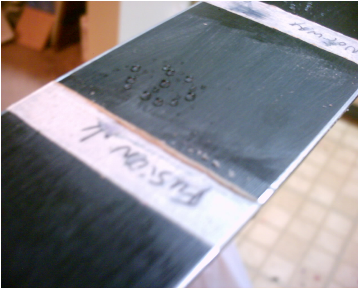
Photo- droplets of distilled water. The droplet broke up upon impact, producing globules. This shows very low surface tension.
